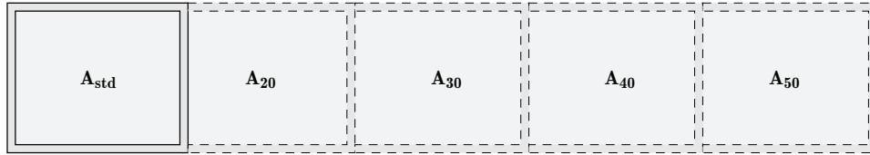
Abbildung 3.1: Bodenplattenvariationen. A_{std} = 10,39m \times 8,65m = 89,93m^2 , A_{20} = 20m \times 8,65m = 173,04m^2 , A_{30} = 30m \times 8,65m = 259,56m^2 , A_{40} = 40m \times 8,65m = 346,08m^2 , A_{50} = 50m \times 8,65m = 432,60m^2 , Aufgrund Außenmaßberechnung \omega_{w,e} = 0m
